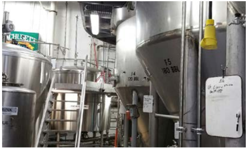
New 50 bbl BrewHouse on left with 120 and 180 bbl Fermenters on right
